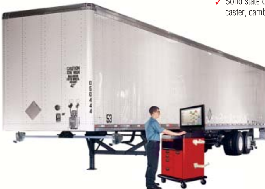
Optional Trailer Alignment Gauge Tool (shown in use with optional DSP506TXF Sensors) mounts sensors to the trailer kingpin. Trailer axles are adjusted to centerline.
